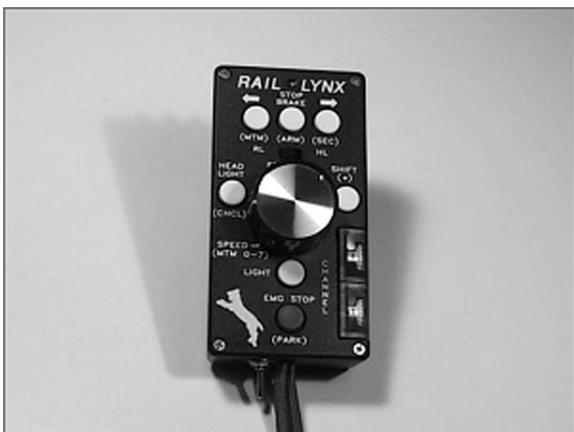
in the direction of the loco. Once a loco receives a command it will continue to do whatever it was last told to do, until it receives another command, or loses power. It is therefore possible to start one train running, change the transmitter channel, and control another locomotive. This is great for demonstrating your railroad to visitors, as you can control multiple locos with one transmitter by simply changing the channel switches.
