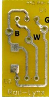
These boards were designed to be a generic aid in mounting and soldering the sensors for in cab installations. Holes for the sensors and for the black, green, and white wires are provided. This is a generic board so a fair amount of flexibility was designed in to allow it to fit most applications.
